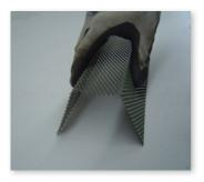
Tile valley product, end view, in squeezed position prior to inserting into tile valley. Once in position release the product & seal along both sides between mesh & tile.
