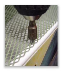
NOTE: Make sure never to over tighten any of the screws. The product only requires positive pressure to secure it in place.
